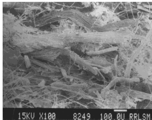
Figure 9 SEM of fracture surface of PALF-polyester composite under flexural failure (fiber content 30 wt %).
